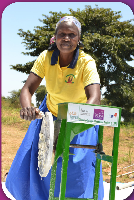
a farmer demonstrates a groundnut shelling machine. This removes the husk from the groundnuts to give you what we know as peanuts.
